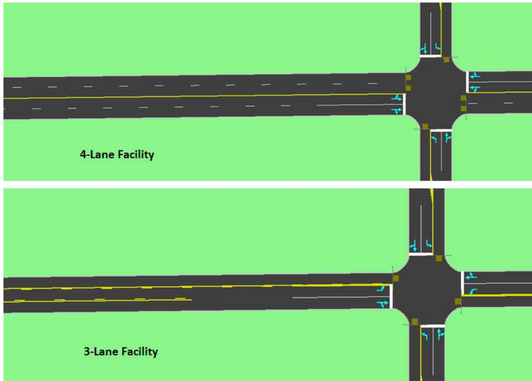
Figure 2: Conceptual Layout of 4-Lane and 3-Lane Roadway
