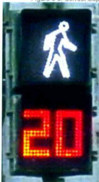
Figure 3-9. Incorrect display because countdown is displayed during WALK interval
