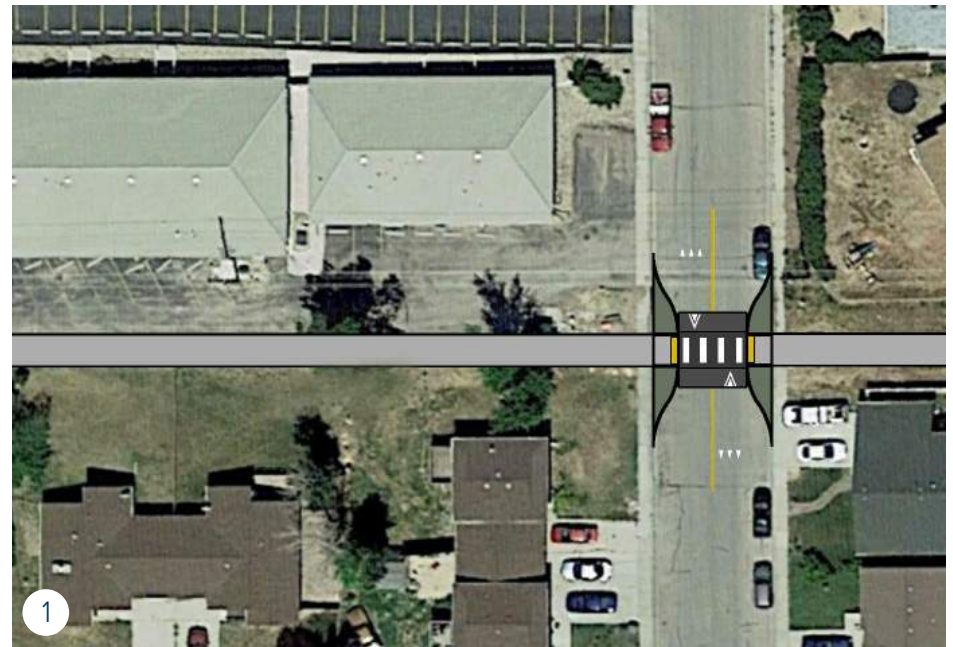
A designated mid-block crossing on Wagonhammer Rd including curb extensions and a raised crosswalk will ensure trail users are highly visible, and will encourage vehicles to slow down and yield to trail users.
