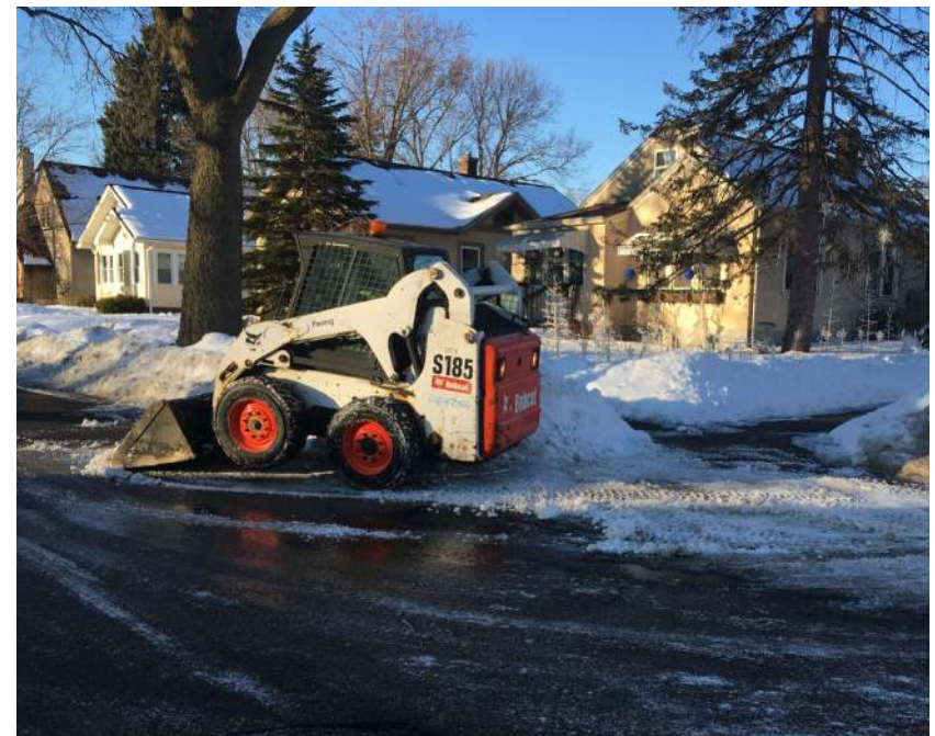
A bobcat with a plow can be used to plow shared use paths and sidepaths.
