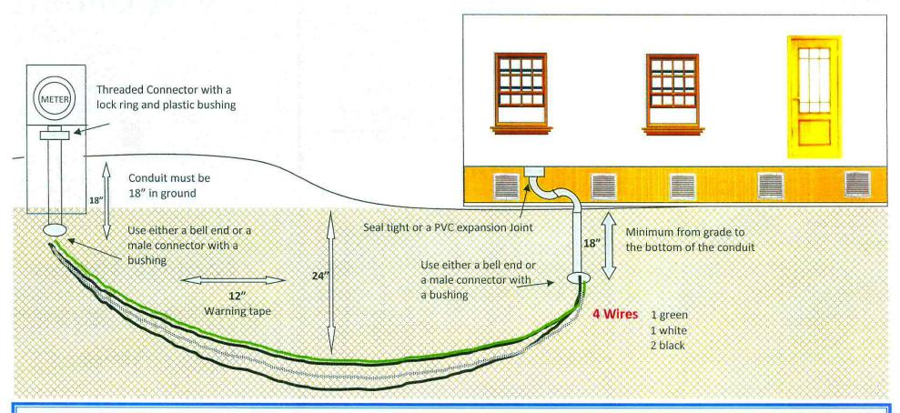
Feeder conductors shall be sized according to the tag on the mobile home. If the tag on the mobile home is more than 50 amperes, then it can not be cord connected.
